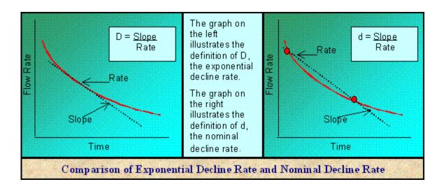
Usually, the nominal decline rate, d, is used when dealing with flow rate data in tabular rather than graphical format. The equivalence of the (true) exponential decline rate, D (as used in the exponential decline equation) and the "nominal" decline rate, d (as used in many hand calculations) is shown below:
