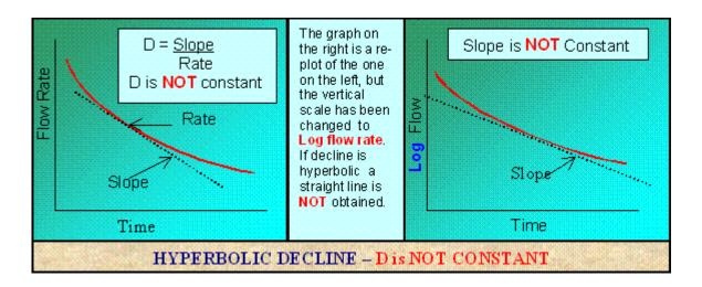
Unfortunately, hyperbolic decline does not plot as a linear relationship on a Cartesian grid. As shown above, plotting "Rate vs. Time" or "Rate vs. Cumulative Production" on semi-log scales does not straighten a hyperbolic decline curve either. Prior to the widespread use of personal computers, this lack of linearity was the main reason for the restricted use of hyperbolic declines.
