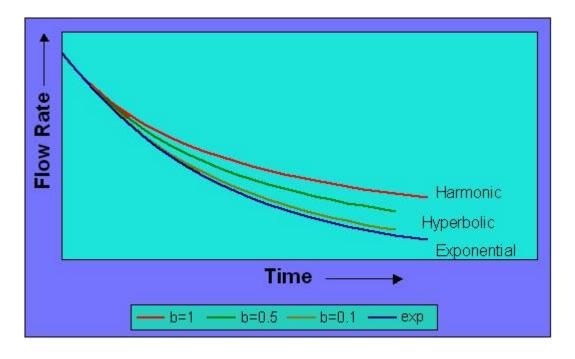
Decline curve analysis is usually conducted graphically, and in order to help in the interpretation, the equations are plotted in various combinations of "rate", "log-rate", "time," and "cumulative production". The intent is to use the combination that will result in a straight line, which then becomes easy to extrapolate for forecasting purposes. The decline equations can also be used to forecast recoverable reserves at specified abandonment rates.
