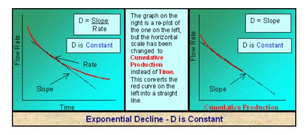
It can be shown mathematically, that an exponential decline will also result in a straight line when plotted as Flow Rate vs. Cumulative Production.
